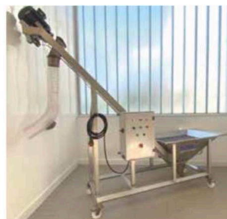
Station vide sacs mobile.
